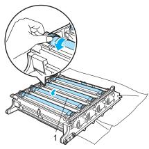
When you have found the mark on the drum that matches the print sample, wipe the surface of the drum gently with a cotton swab until the dust or paper powder on the surface comes off.
